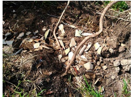
Image 18: Unearthed asbestos debris
