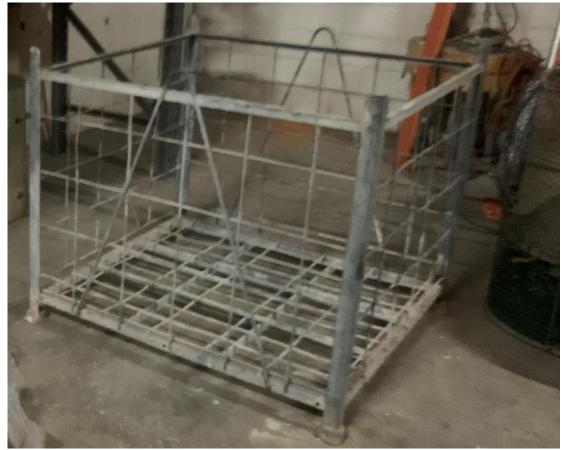
Image: The mesh storage cage used was not a suitable forklift workbox.
