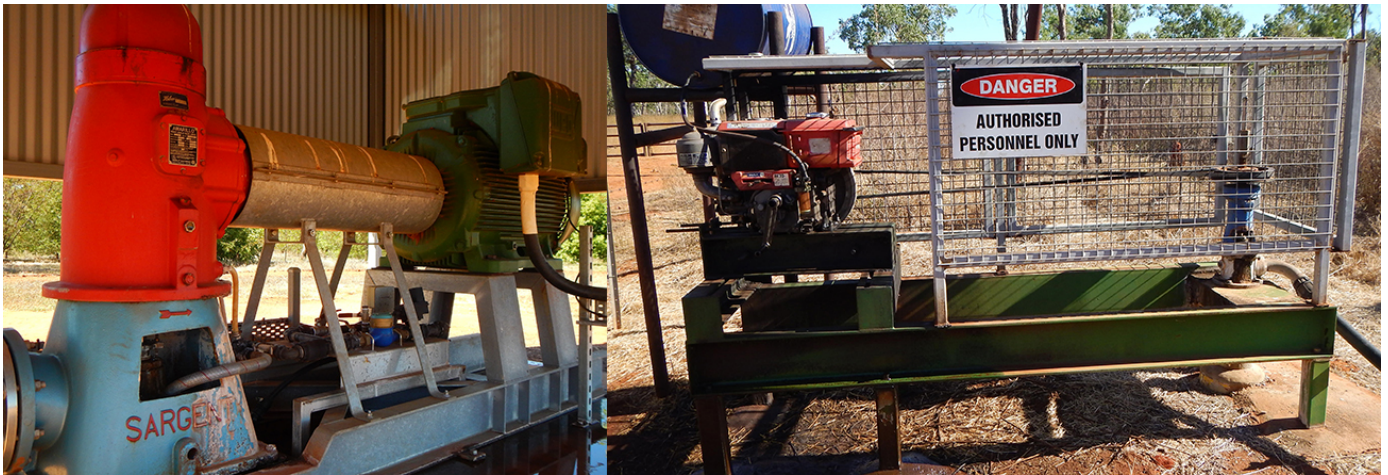
Image 2: Two examples of bore pumps fitted with guards. (Source: Dept. of Environment Parks and Water Security)
