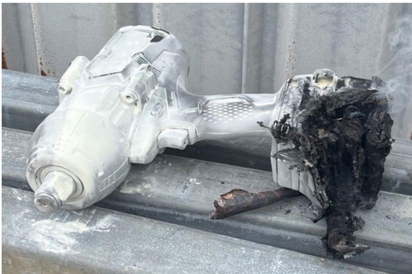
**Image:** The still smoking lithium-ion battery after being extinguished by a dry power extinguisher.
