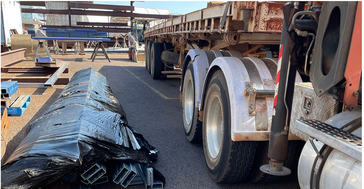
Image: The worker was standing beside the trailer when the bundled steel slipped from the forklifts tyne.
