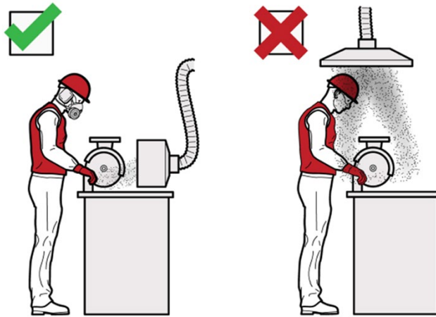
Figure 6: Examples of using local exhaust ventilation
