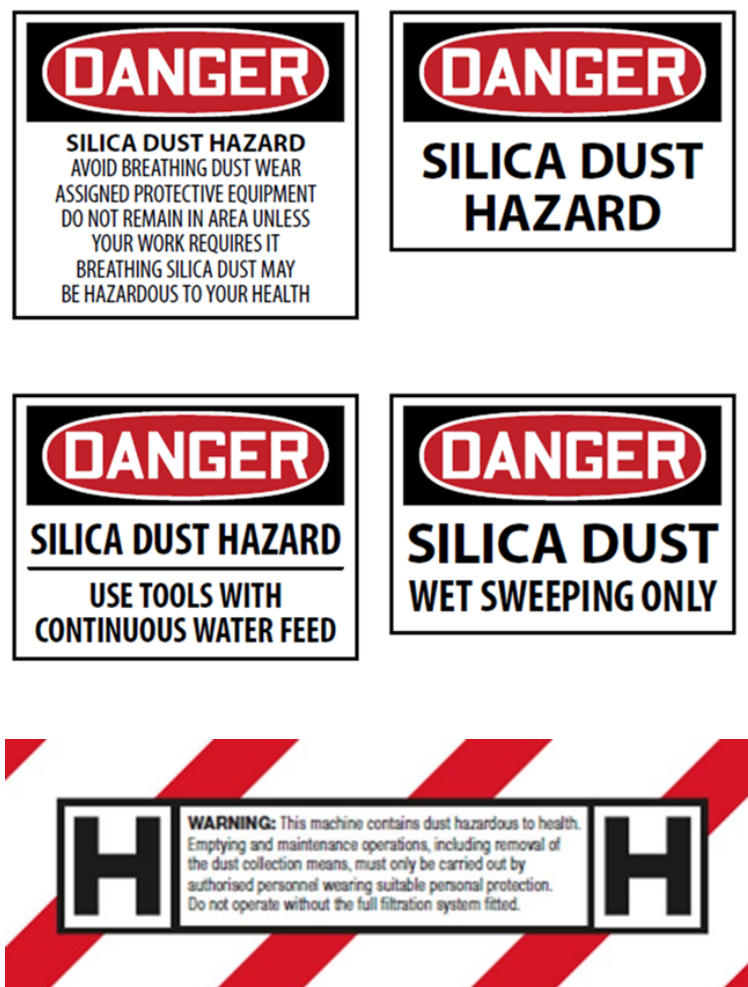
Figure 3: Examples of dust hazard signs
