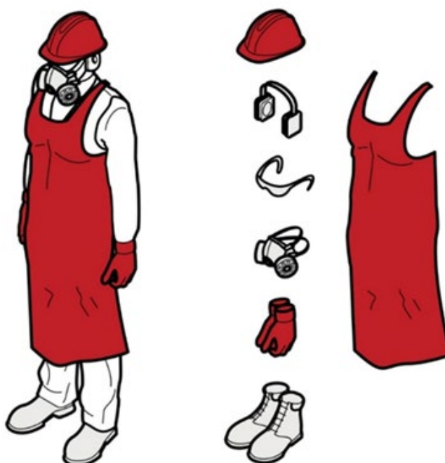
Figure 4 Examples of personal protective equipment
