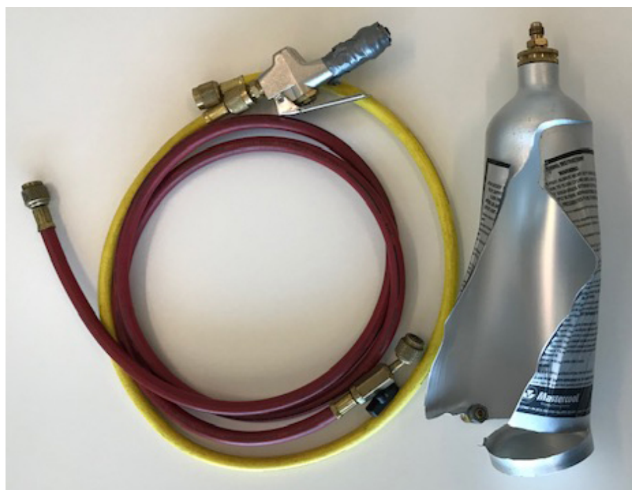
Image 1: Over pressurising canisters will cause it to rupture.
