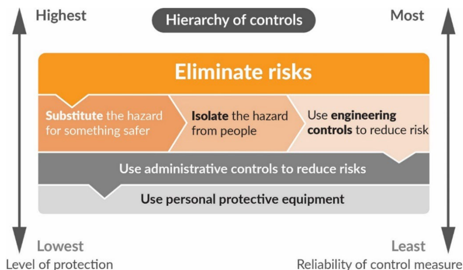
Figure 3: The hierarchy of controls
