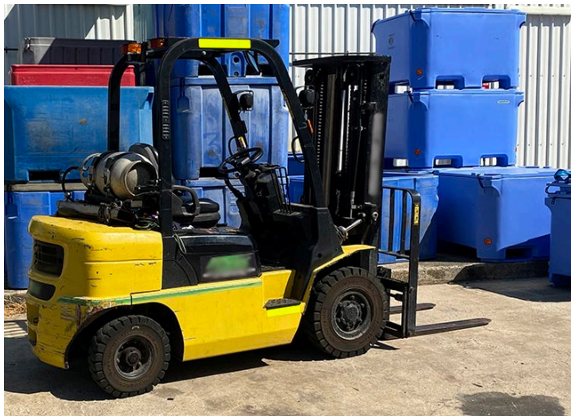
Image: The fuel-powered forklift should not have been used in an enclosed space.
