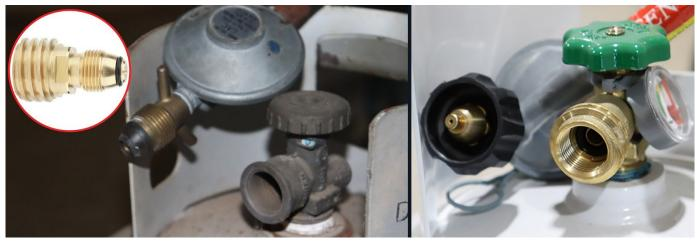
**Image:** Type 21 POL appliance connector and cylinder connection (left) and LCC27 appliance connector and cylinder connection, which has both internal and thicker external threads (right). The insert image shows an aftermarket adaptor, which should not be used.
