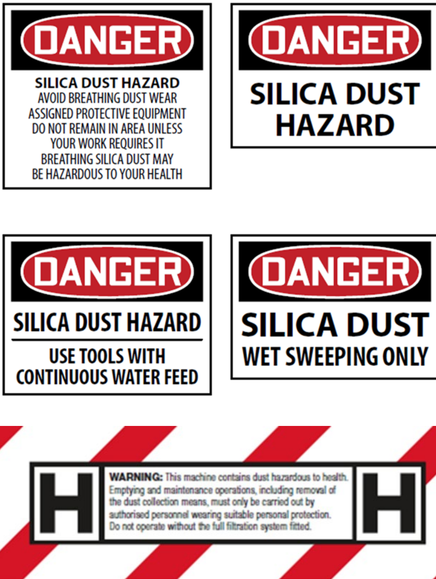
Figure 4. Examples of dust hazard signs
