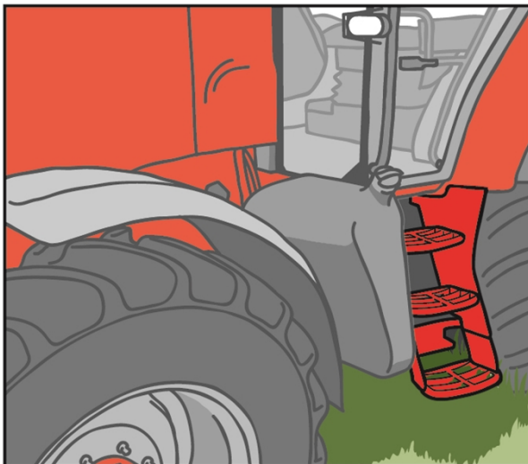
Figure 3 Tractor access platform
