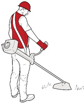
Figure 32 Weight supported by a harness; heaviest part of the brush cutter located behind the wrists
