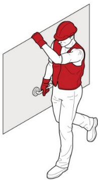
Figure 27 Use handling grip devices adapted to the particular object to be carried
