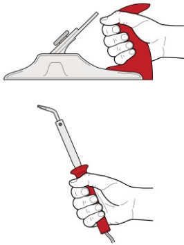
Figure 28 Select tools that can be held with a neutral wrist or in a handshake position with the hand adopting a comfortable, not too open or too closed, grip. Orient jigs and fixtures holding the work piece so the wrist does not have to bend.
