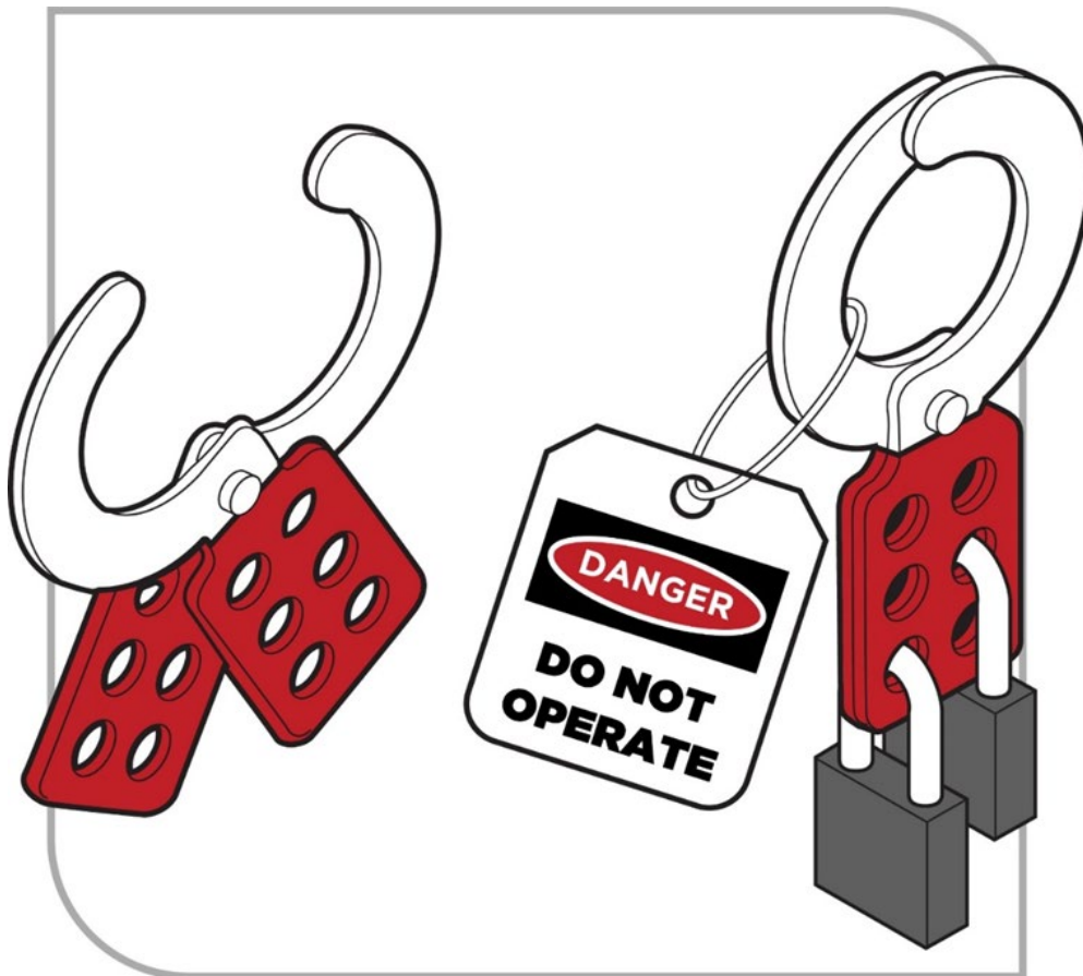
Figure 3 Example of tag and lockout with padlocks
