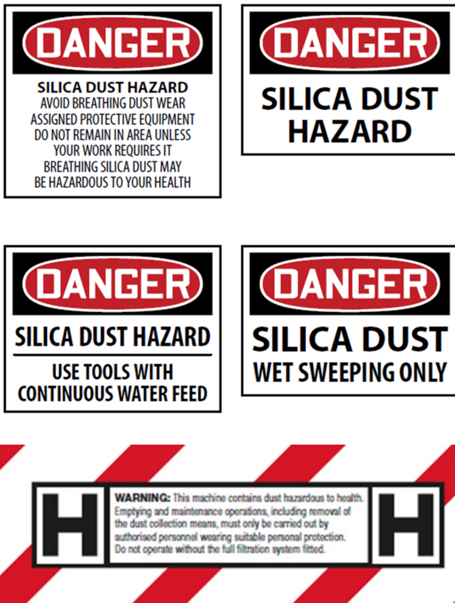
Figure 4. Examples of dust hazard signs
