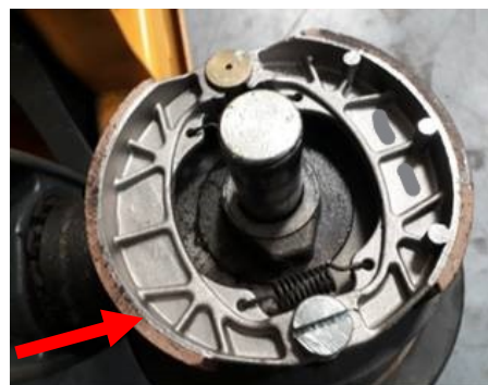
Figure 1: Uncovered brake assembly of an affected manual hand pallet truck
