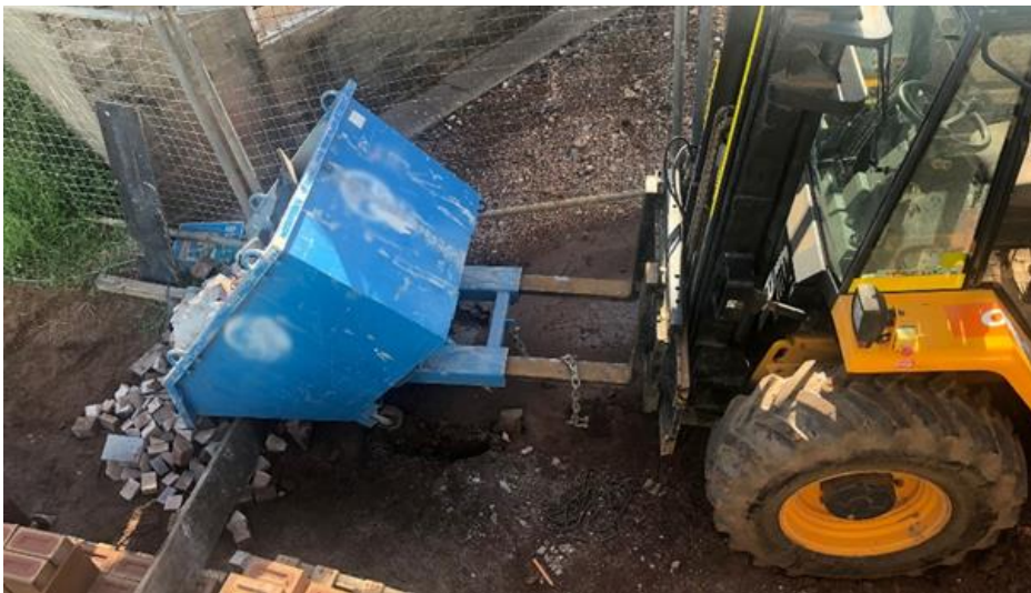
Image 1: The forklift tines were not fully inserted into the bin pockets.
